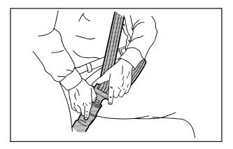
To unlatch the belt, push the button on the buckle. The belt should go back out of the way. When the safety belt is not in use, slide the latch plate up so that it is stored on the safety belt stitching, near the guide loop.
